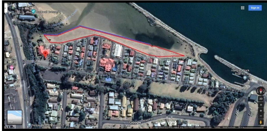
Image 3 – shows the area of reclaimed land to the north of the existing road. The temporary revetment wall (blue) is visible along the waterfront boundary. Photo courtesy of Google Images.
